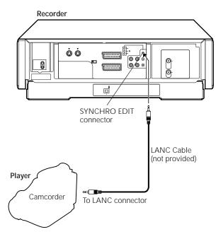
The Synchro Editing function synchronizes the start of the playback and recording operations when starting an edit operation using a camcorder with LANC connector and your video recorder.
